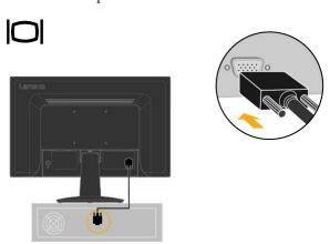
3. Plug in the monitor power cord and the computer cord into grounded electrical outlets.
