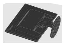
Step 3: Remove the base and stand from the monitor, refer to "Detaching the monitor base and stand" on page 2-7".
